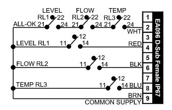
Signals are accessible via a standard two-row 9pin D subminiature connector. See image to the right; the female gender (ATC PN EA096) is supplied in all cases. If male pins are required, we recommend using a male-to-male gender-changer connector. Pin numbers are clearly marked on the molding. The connector is rated to IP67.
