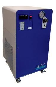
The A02 Airblast chiller is housed in a G02/K02 enclosure. It has a low footprint, taking up less space on factory floors. Taller than previous ATC designs, the A02 allows for the integration of centrifugal pumps, which require head pressure to prime correctly. The A02 is available on singlephase, from 208 to 240V.
