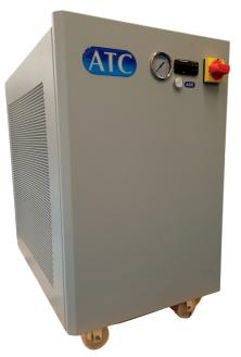
The A08 is housed in a K6 enclosure, a versatile option with lots of space for additional options to be installed. It is suitable for use with both centrifugal and positive displacement pumps. The A08 is available in single- and three-phase configurations. There are two twin heat exchangers within the A08, providing some redundancy among the four fans if ever one was to fail. This makes the A08 a good unit for processes that cannot be interrupted.
